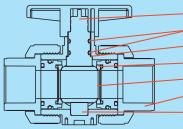
Large diameter shaft eliminates breakage
