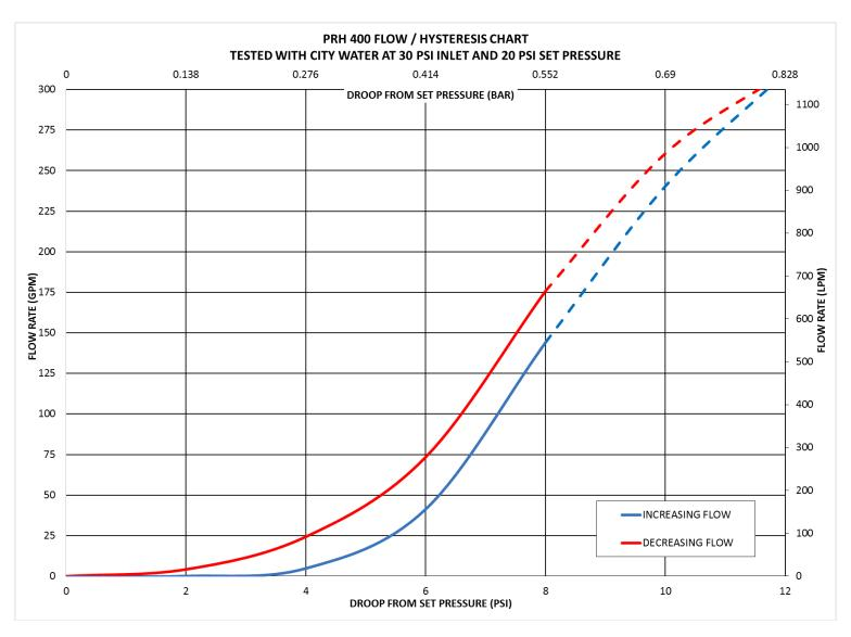
NOTE: Dashed lines in curves above exceed the recommended maximum flow rate of 5 feet per second for thermoplastic piping.
