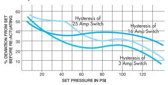
Deadband helps to prevent oscillation or "hunting". In other words, without sufficient deadband, the switch will be actuating and de-actuating too often. For applications where it is critical to de-actuate with less deadband, a 3 Amp switch is available. See specifications below.
