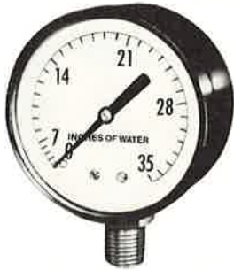
DIAMETER: 2-1/2" DIAPHRAGM: Beryllium copper MEASUREMENT: 0-35" H 2 O PART NUMBER: W35
