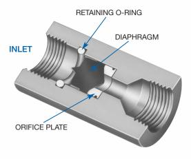
Single diaphragm design at left used for ¼ GPM through 8 GPM (.95 LPM - 30 LPM) constant flow rates. All higher flow rates use multidiaphragm design (consult factory for availability).
