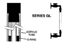
Series GL typical installation includes two ball valves (not included) for easy service. Overlap sighting area for continuous level indication with no visual dead spots. Do not series connect GL with pipe nipples because the assembly will be unstable and a visual dead spot will be created.
